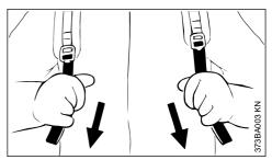
Pull the ends of the straps downward to tighten the harness.
