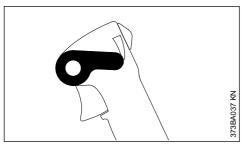
► Move the setting lever to the idel position.
