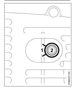
If the engine power is decreasing or does not run smoothly at maximum RPM, check the spark arresting screen (not available in all versions) in the muffler.
