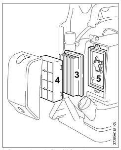
Remove the main filter (3) from the cover and inspect it – if it is dirty or damaged, fit a new one.
