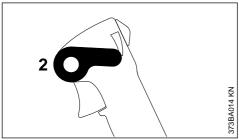
► Move setting lever (2) to lower stop – the engine settles down to idle speed.
