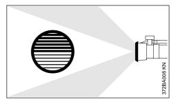
Splits the spray jet in two – allows two closely planted rows to be treated in one pass.
