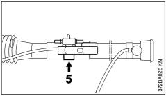
► Tighten down the clamp screw (5) (see "Adjusting the Control Handle").
