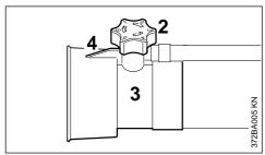
► The discharge rate can be infinitely varied by turning the metering knob (2) on the nozzle (3).
