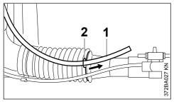
Secure liquid hose (1) from the container to the pleated hose with the retainer (2).
